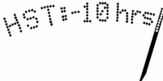
Figure 4: Display after switching to HST
