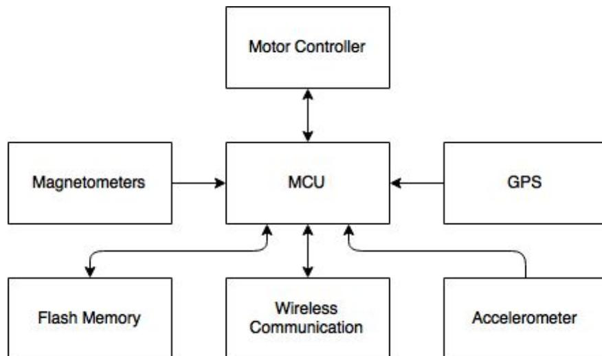
*Figure 2: Block diagram of hardware communication signals*
