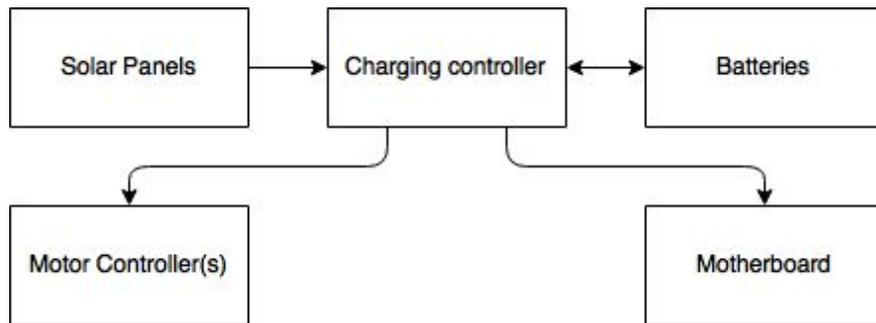
*Figure 1: Block diagram of power distribution*
