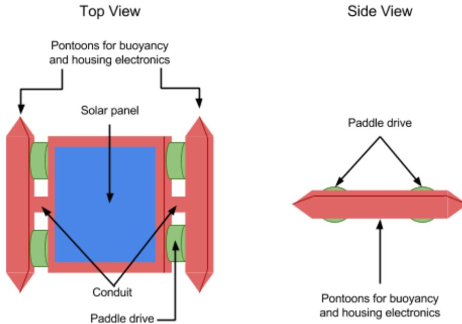
Figure 4: *Diagram of potential chassis of drone (not to scale)*
